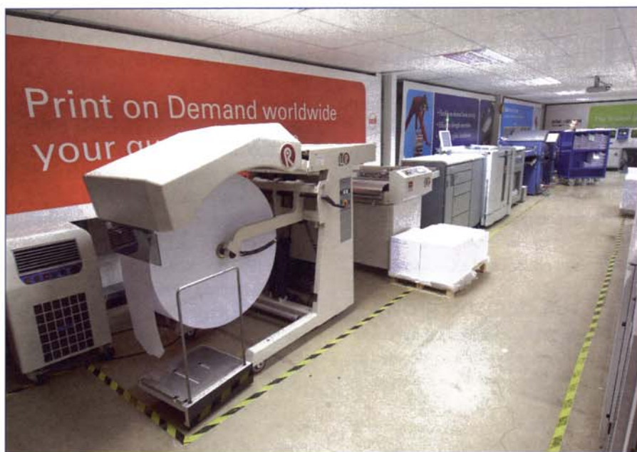
The roll fed VarioPrint 6320 line, with the blue MBO finishers just visible at the end.
